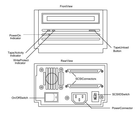
Figure 1–1 Model TLZ07-DA (Tabletop - Original Version)
