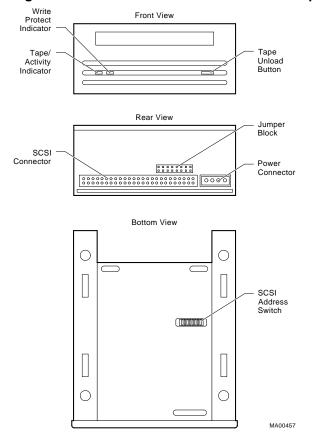
Figure 1–4 Revised Version TLZ07-AA/-BA Tape Drive
