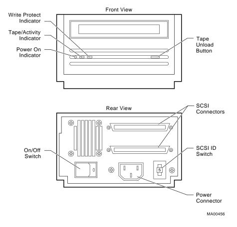
Figure 1–2 Revised Version TLZ07-DA Tabletop Tape Drive
