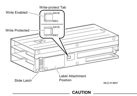
The write protection status of the magazine is determined by checking the reflective plate on the write-protect tab. In order to ensure correct determination of the status, keep the plate reasonably clean, and never affix labels or the like over the write-protect tab.
