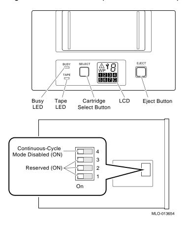
Figure 7–1 Model TLZ9L-AA (Front and Bottom View)
