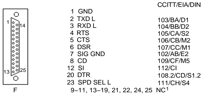
Figure 9-1 25-Pin Port Pin Numbers
