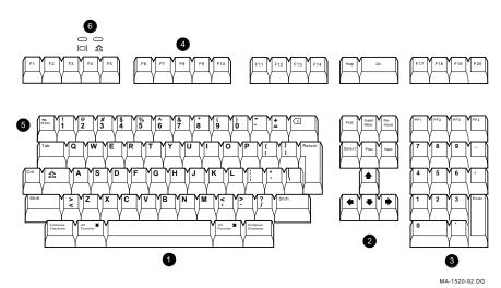
Figure 1–1 DEC VT-Style Keyboard Layout
