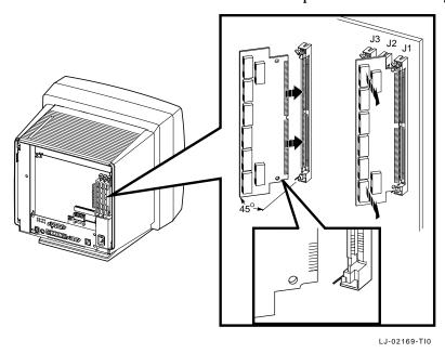
**VX227 model:** If there is an image accelerator board installed to the left of slot J3, temporarily remove the image accelerator board before trying to install a memory module in slot J3.
