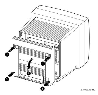
To close the VX225 cover, press in the two locking tabs **1** with your thumbs and push the cover into place. Release the tabs to lock the cover in place.
