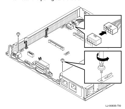
7. Disconnect any cables connected to the logic module through the rear panel.
