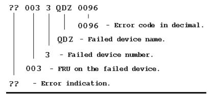
Table 4–1 lists possible error codes. The probable solution for any error code not listed in the table is to replace the system logic module. To display a complete list of all the devices in the terminal's configuration, enter the  $\tt SHOW$  CONFIG console command.
