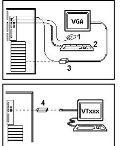
Figure 2-4 Connecting a {XE "Graphics option slot"}Monitor or Terminal
