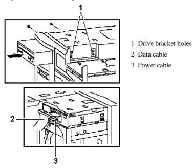
Figure 5-12 Installing a CDROM Drive
