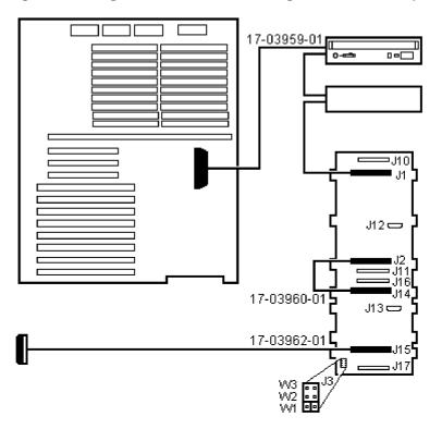
Figure 6-8 Single-Controller SCSI Configuration with Jumper Cable
