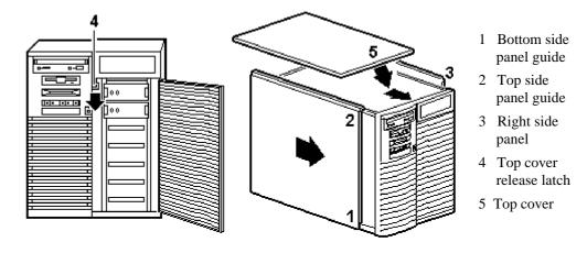
Figure 5-3 Replacing the Top Cover and Side Panels
