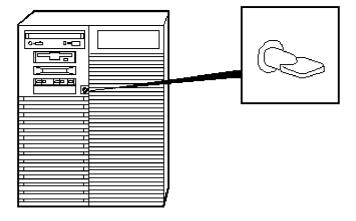
Figure 2-7 System Lock and Key
