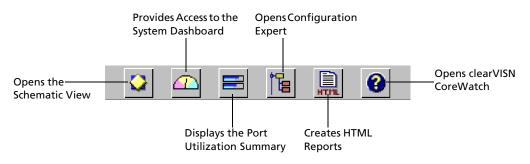
Figure 6. clearVISN CoreWatch toolbar buttons
