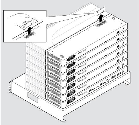
Figure 11-3: Stack Interconnect Card Removal
