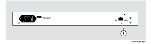
The setup port on the Stack Station (1) is used to set initial configuration parameters in an unmanaged stack.
