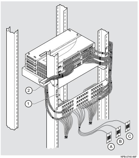
Action Step 1 Secure the mounting flange (1) on the tray to the mounting rails of the standard 19" rack using the mounting screws. 2 Attach the cable harness bracket (2) and office attachment connectors A, B and C.
