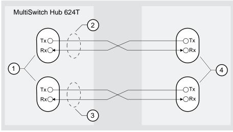
Figure 5-1: Simple Redundant-Link Configuration
