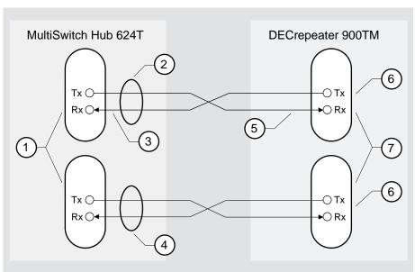
Figure 5-3: Partial Fault Detection Configuration
