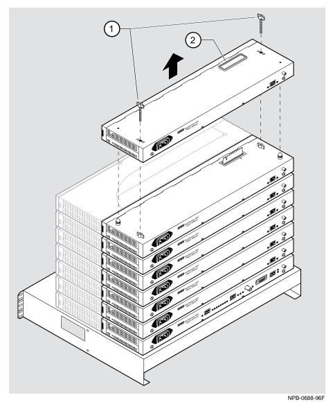
11-4 Removing or Replacing a Level on the Stack
