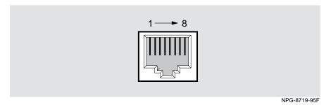
Table B-1: 10BaseT (8-pin MJ) Connector Pin Assignments
