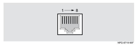
**Table B-5: Stack Director and Stack Station Setup Port Connector Pin Assignments**
