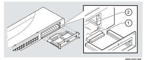
Step Action 1 Make sure that power to the DIGITAL MultiSwitch Hub 624T is off by unplugging the module from its DIGITAL MultiSwitch 600 System or DEChub 900 MultiSwitch. 2 Loosen the four screws and remove the dust cover from the module's expansion slot. 3 Hold the DIGITAL MultiSwitch Hub 624T Carrier Card by its bezel and align its edges (1) with the card guides (2) in the module's expansion slot. Push the Carrier Card into the slot until it is firmly seated inside the module.
