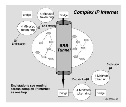
Figure 3–1 Example of the Bridge Tunnel Feature
