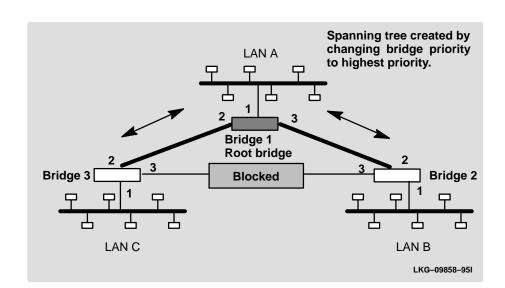
Figure 2–3 **User-Adjusted Spanning Tree**
