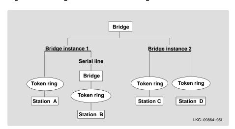
Figure 2-9 **Bridge Instances Within a Bridge**
