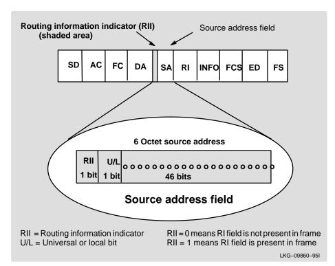
Figure 2–5 802.5 Source Address Format
