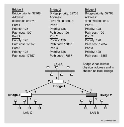
The spanning tree algorithm designates the port connecting Bridge 1 to Bridge 3 (port 2) as a backup port and blocks it from forwarding frames that would cause a loop condition. The spanning tree created by the algorithm using the default values is shown in the Figure 2–2 as the heavy lines connecting Bridge 1 to Bridge 2, and then Bridge 2 to Bridge 3. The root bridge is Bridge 2.
