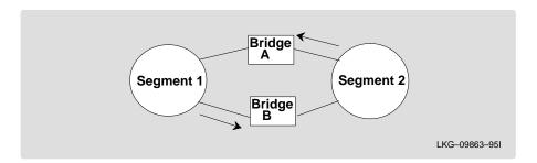
Note: For source routing to work, some end-node applications such as the IBM PC LAN program require you to enable spanning tree explore on attached interfaces. For parallel bridge configuration, the spanning tree explore option should be enabled only on one of the parallel interfaces. No serious harm (other than some extra traffic) results from having too many interfaces enabled for the spanning tree.
