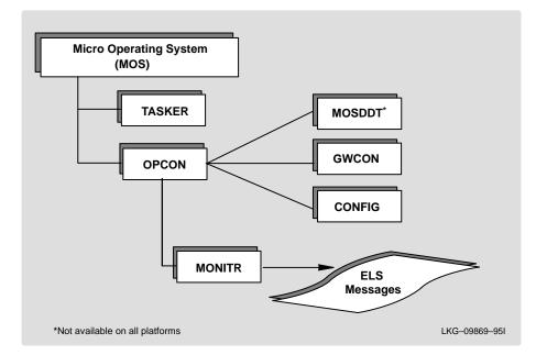
Figure 1–1 Router Software Processes
