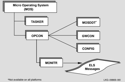
The CONFIG interface contains commands that let you configure and monitor interfaces and protocols. Each command has its own prompt. For example, the prompt for the TCP/IP protocol is IP config>.
