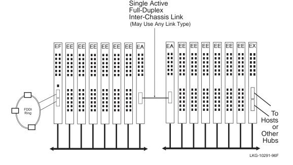
Though not shown in this figure (or in Figure 4-23), more than two parallel links can be configured. For example, two VNswitch 900EA modules could be used in each hub to provide full-duplex links for multiple VLANs, with a separate bridge tunnel configured for each VLAN. In this case (using VNswitch 900EA modules), the dual full-duplex links would provide approximately 620 Mb/s of inter-chassis capacity (155 Mb/s in each direction per link).
