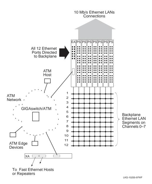
Figure 4-12: Low-Throughput ATM Switching Example
