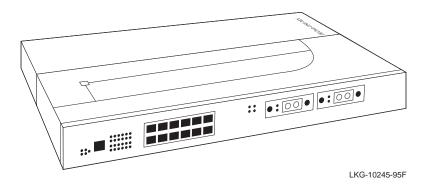
The unit is auto-configured to connect to the 400 Mb/s VNbus, which provides interoperability across the backplane with other VNswitch modules while maintaining front panel connectivity. Additionally, each of the module's 12 front-panel 10BaseT 802.3/Ethernet ports can be individually redirected to a MultiSwitch 900 backplane LAN segment to create a backplane LAN. Also, port 12 can be redirected to the MultiSwitch 900 backplane ThinWire LAN segment.
