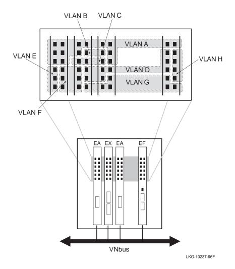
Another important function of the VNbus is to allow a VNswitch module that has its routing software enabled to serve as a router for one or more other VNswitch modules in the hub, as shown in Figure 3-11.
