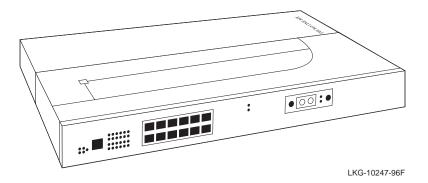
The VNswitch 900EA module has twelve 10BaseT Ethernet switched ports on the front panel and a single high-speed ATM port. The ATM port incorporates as many as 16 logical ports (as described in the section on ATM Features in Chapter 3).
