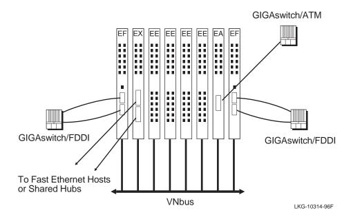
In this configuration, all the VNswitch modules are connected to the same VNbus, illustrating how all four technologies can co-exist in the same network. For example, when the modules are configured into a single VLAN (the default VLAN), the LANs attached to the VNswitch ports function as a single LAN, allowing information to flow freely between all attached devices regardless of the different LAN technologies used.
