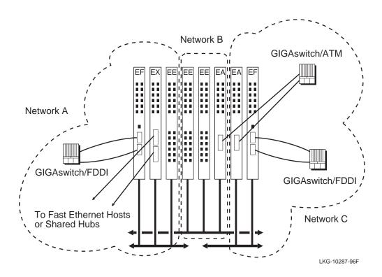
In Figure 4-22, the VNswitch routing software provides routing between VLANs that reside on one or more modules attached to the same VNbus. In this illustration, three modules (one from each cluster, or network) are configured with the routing software enabled. More modules can be configured with the routing software enabled if additional capacity or redundancy is needed.
