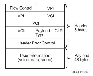
An ATM cell is broken into two main sections, the header and the payload.
