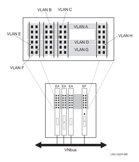
By default, all ports (including the high-speed ports) on the VNswitch modules are grouped into a single VLAN, called the *default VLAN*. Through software commands, the ports can be arbitrarily divided into port groups (as shown in Figure 3-37). Any ports not included in a port group (or VLAN) remain in the default VLAN. Thus, the high-speed ports in this illustration are all members of the default VLAN.
