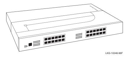
All of the module's 24 front panel 10BaseT 802.3/Ethernet ports are auto-configured to connect to the 400 Mb/s VNbus on the MultiSwitch 900 backplane. Additionally, as many as 12 of the ports can be individually redirected to a MultiSwitch 900 backplane channel (LAN segment) to form a backplane LAN. Also, port 12 can be redirected to the MultiSwitch 900 backplane ThinWire LAN segment.
