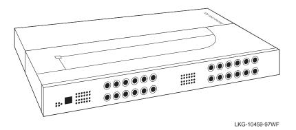
All of the module's ports are auto-configured to connect to the 400 Mb/s VNbus on the MultiSwitch 900 backplane. Additionally, the module's 12 backplane ports can be individually directed to a MultiSwitch 900 backplane channel (LAN segment) to form a backplane LAN. The module's backplane port 12 can be connected to the MultiSwitch 900 backplane ThinWire LAN segment.
