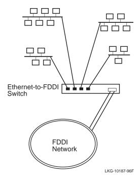
The VNswitch family includes an Ethernet-to-FDDI switch called the VNswitch 900EF. The VNswitch 900EF is an Ethernet-to-FDDI switch that can connect multiple LANs to an FDDI backbone or network. The VNswitch 900EF features a single-port pair (DAS or SAS) FDDI interface and twelve 10BaseT ports.
