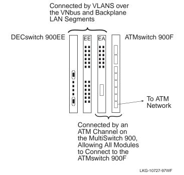
As shown in Figure 3-36, this feature also allows earlier DEChub modules (such as the DECswitch 900EE) to connect to an ATMswitch 900F.
