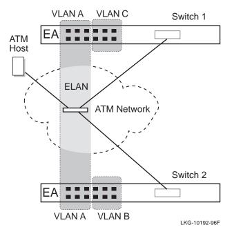
As many as 16 emulated LANs (ELANs) are supported on each VNswitch 900EA, XA, and FA module. Each ELAN may consist of VLANs that span multiple modules in the hub, allowing LANs from the VNswitch 900EE, EX, XX, or EF to be joined with LANs on other VNswitch modules residing in a separate hub on the other side of an ATM network. Refer to Figure 1-19.
