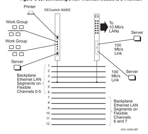
Figure 3-30: Connecting a Non-VNswitch Module to a VNswitch
