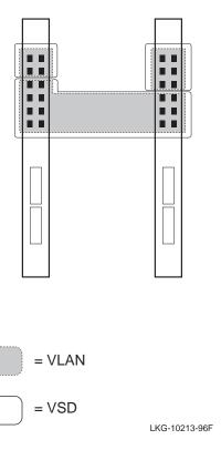
Since only port-based (Class 1) VLANs are supported in Version 2.05, and a VSD consists of a single set of ports (just like a port-based VLAN), the terms VSD and VLAN are sometimes used interchangeably. However, it is important to distinguish between a VLAN and VSD because future versions of the VNswitch firmware may support multiple VLANs per VSD (including VLANs based on ports and protocol type), with features such as overlapping VLANs.
