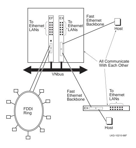
Figure 1-16: Two VNswitch Modules Connected Over a VNbus
