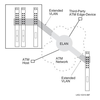
As illustrated in Figure 3-40, a VLAN comprised of ports from three different VNswitch modules in a MultiSwitch 900 is grouped with a VLAN on a standalone VNswitch 900EA switch attached across an ATM network. This is accomplished by
