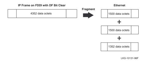
Note that IP fragments are generated only when the IP fragmentation option is enabled (by the management software), the Don't Fragment (DF) bit in the IP header is set to Clear, and the IP header is error free.
