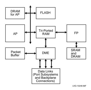
Figure 3-1: VNswitch 900 Series Main Board Architecture
