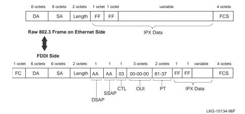
When the switch receives an 802.3 frame while DSAP filtering, it checks the frame's DSAP and SSAP fields. If the field values are FF-FF (indicating a raw IPX frame), the switch generates a SNAP encapsulated frame on the FDDI with PT of 81-37 (Ethernet protocol type for IPX).
