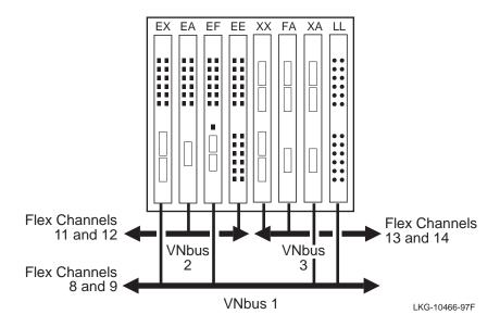
As shown in Figure 3-8, three distinct VNbuses are supported. The VNbuses are physically isolated from each other and each forms a separate network.
