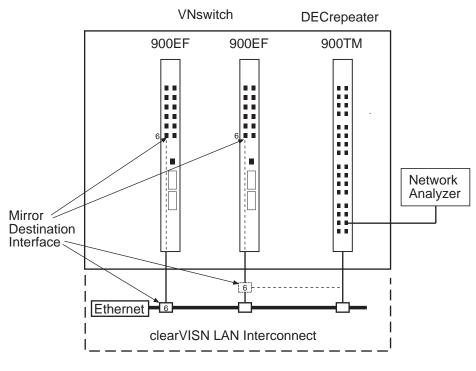
Figure 13-1: Using clearVISN to Connect a Mirror Destination Interface
