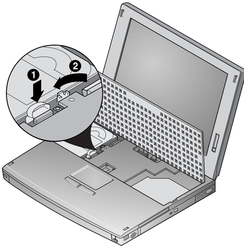
Figure 6-7 Locking the Hard Drive
