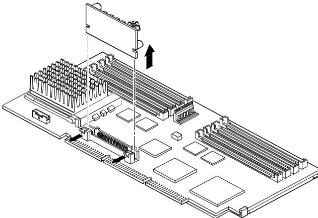
Figure 3 - 25 Voltage Regulator Card
