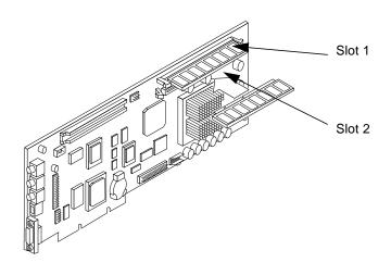
$\textbf{FIGURE 1} \qquad \text{Locating DIMM Slots on the SunPCi Card}$
