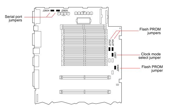
Jumpers are marked on the main logic board with identification numbers. For example, the UPA clock divide jumper is marked J3001.
