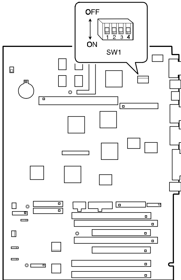
Figure A-1. Main Logic Board Switch Locations
