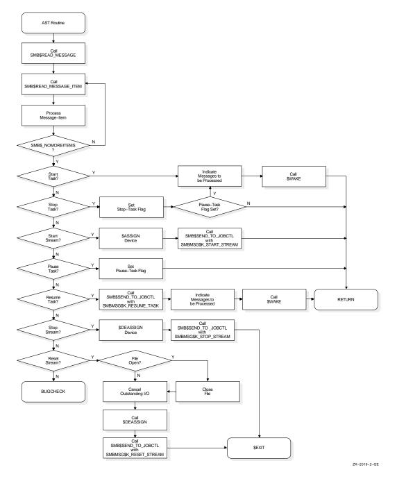
Figure 17–4 Flowchart for a Single-Threaded, Asynchronous Symbiont (AST Routine)
