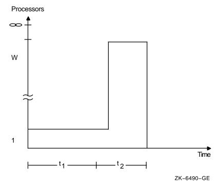
Figure 5–3 shows a typical multiprocessing system, where you have W parallel tasks running on N processors. For this type of configuration, the total processing time  $T_N$  is as follows:
