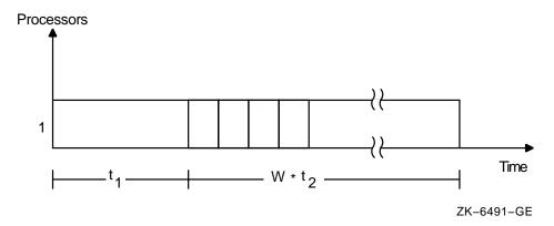
Figure 5–2 shows an application with W parallel tasks being run on a system with an infinite number of processors. Because there are an unlimited number of processors available, no matter how many parallel tasks there are, the total processing time  $T_{\infty}$  is as follows:
