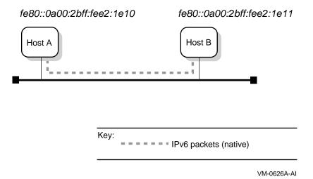
Figure 1–11 shows a simple LAN configuration in which host A, host B, and router A communicate using IPv6. Host A and host B obtain global addresses from router A.
