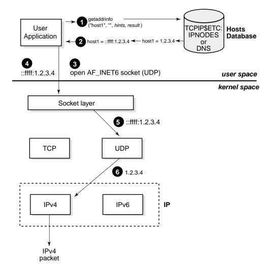
Figure 7–2 Using AF\_INET6 Socket to Send IPv4 Communications
