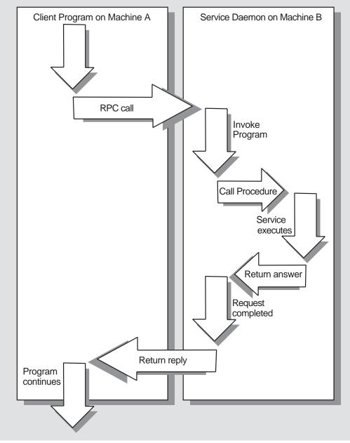
Figure 1–1 Basic Network Communication with Remote Procedure Call
