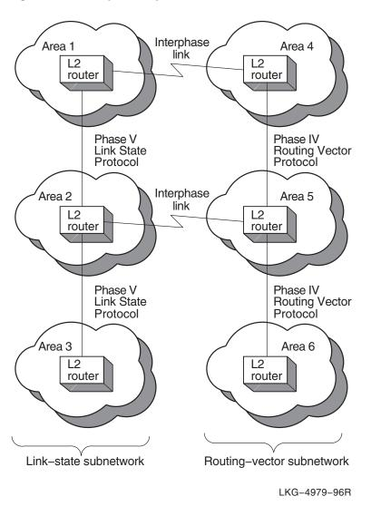
Figure 4–5 Multiple Interphase Links Between Two Subnetworks
