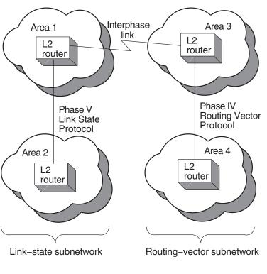
Figure 4–2 Configuration Requiring Manually Created Interphase Links
