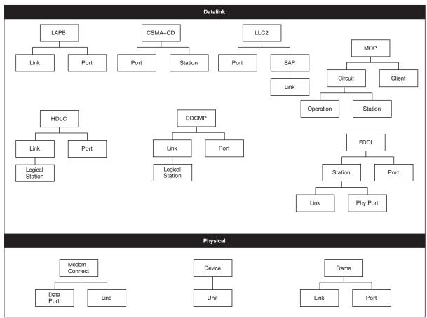
Figure 1–4 Entity Hierarchy and the Lower Layers
