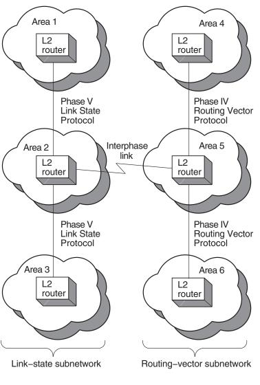
Figure 4–4 Single Interphase Link Between Two Subnetworks
