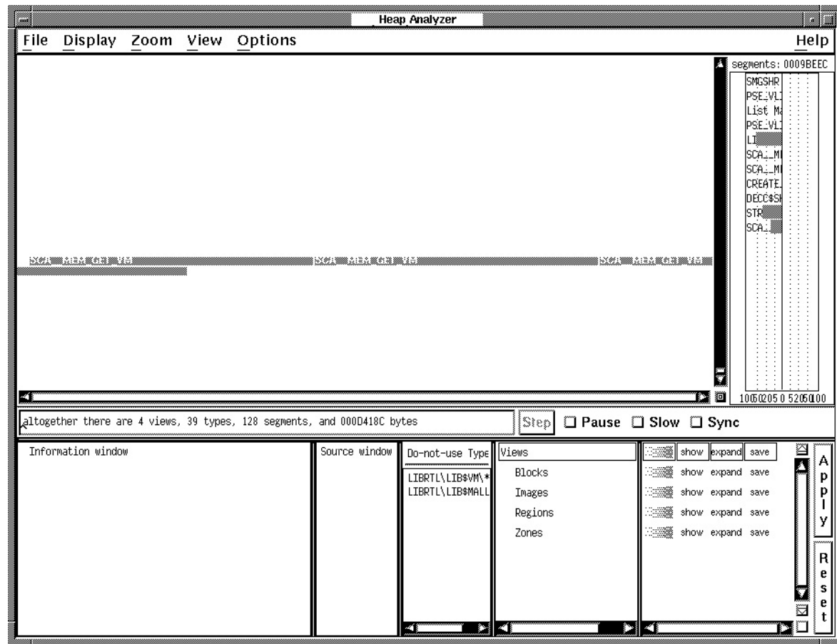
Figure 12–12 Incrementing Memory Allocation Indicates a Memory Leak
