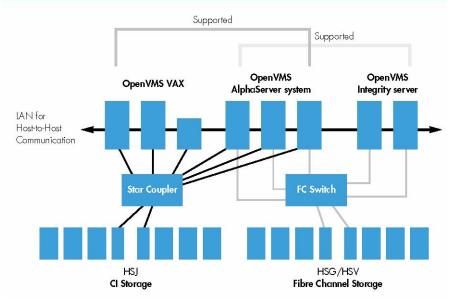
Figure 3 – OpenVMS cluster with VAX, Alpha, and HP Integrity servers (from *The HP OpenVMS Approach to High Availability Computing*, July 2004)
