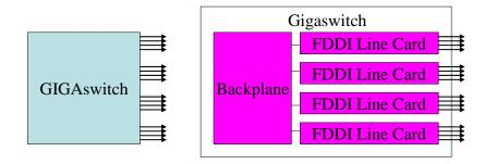
port each LAN adapter is connected, then failure reports will be able to identify failures down to the line card level and even to the individual port level. The Level of Detail Example shows, on the left, a GIGAswitch represented as a black box, and, on the right, a GIGAswitch represented as line cards and the backplane connecting them in the box.
