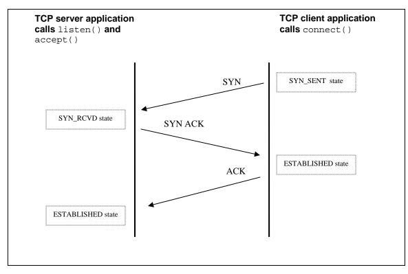
Figure 2 TCP Connection Establishment - "Three-Way Handshake"
