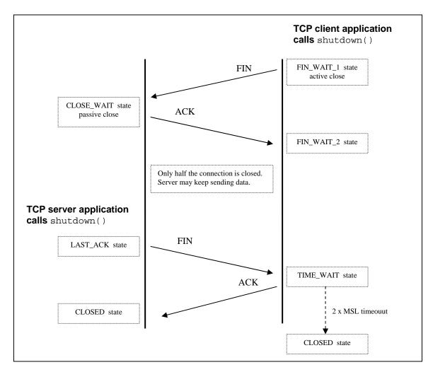
Figure 3. Closing a Connection - 4-Way Handshake
