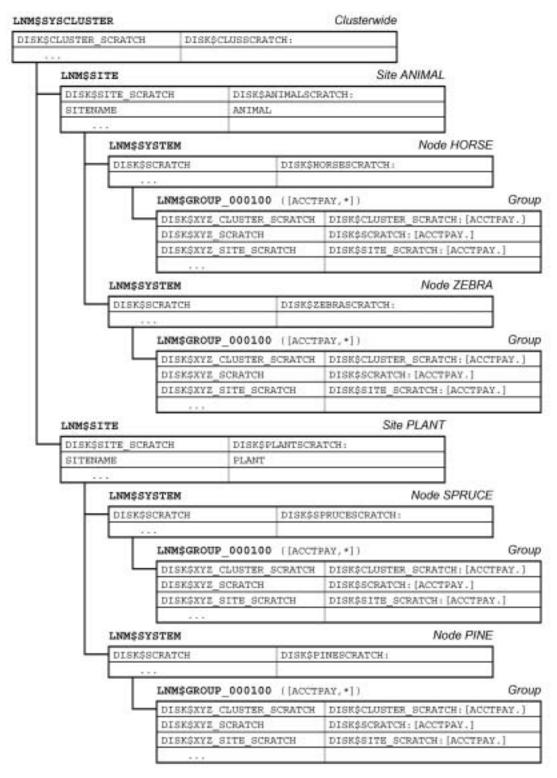
Figure 4 – Inheritance with rooted, concealed logical names.
