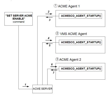
Figure 3: ACME Control Flow for ACME\$CO\_AGENT\_STARTUP
