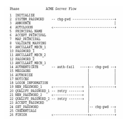
Figure 4: Authentication and change-password request phases and flow
