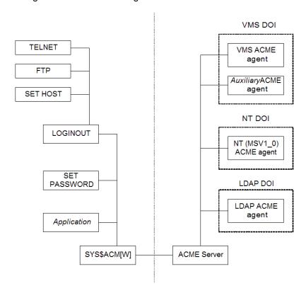
Figure 1: Overview of the ACME Subsystem
