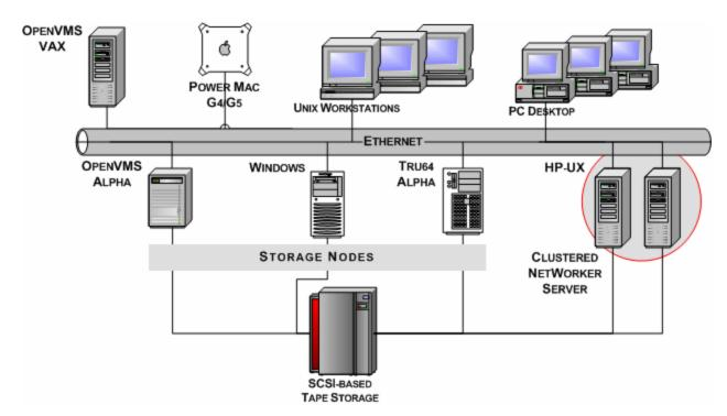
Figure 1: A Typical NetWorker Environment, with SCSI-Based Library Sharing
