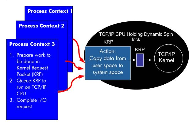
Figure 3 Process Context Threads in the Scalable Kernel
