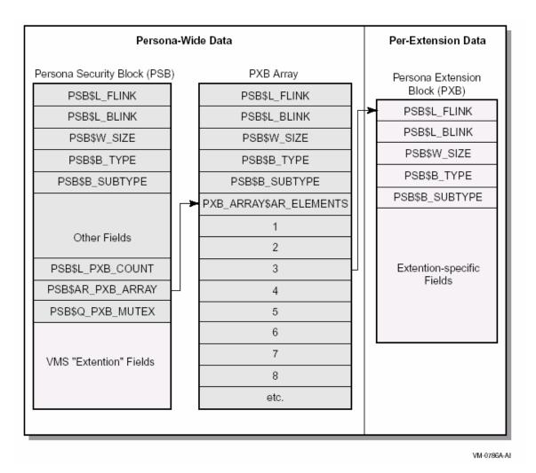
Figure 7: Some persona data structures (credentials are stored in "Extension-specific Fields")
