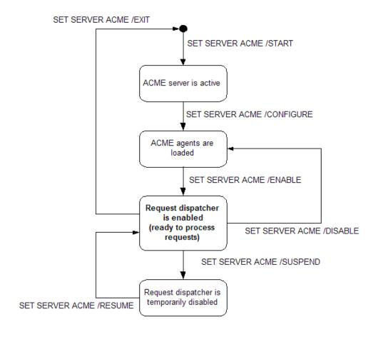
Figure 5: SET SERVER ACME commands and states of the ACME subsystem
