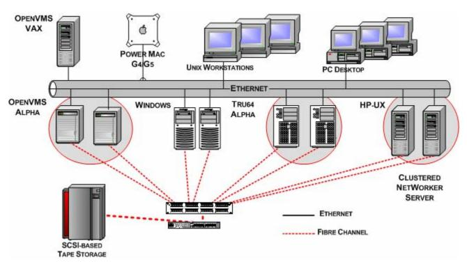
Figure 3: Sharing tape resources on a SAN with DDS. Tape devices within a shared library are not allocated to an individual server. The NetWorker Server and each Storage Node can utilise any available tape device.
