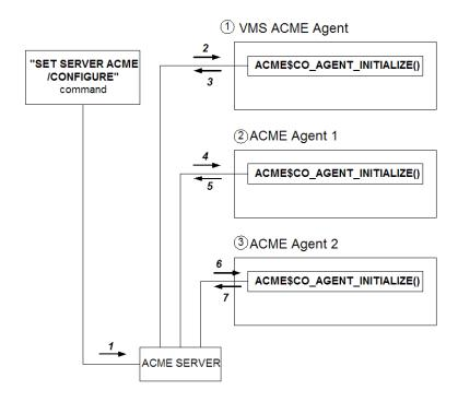
Figure 2: ACME Control Flow for ACME\$CO\_AGENT\_INITIALIZE
