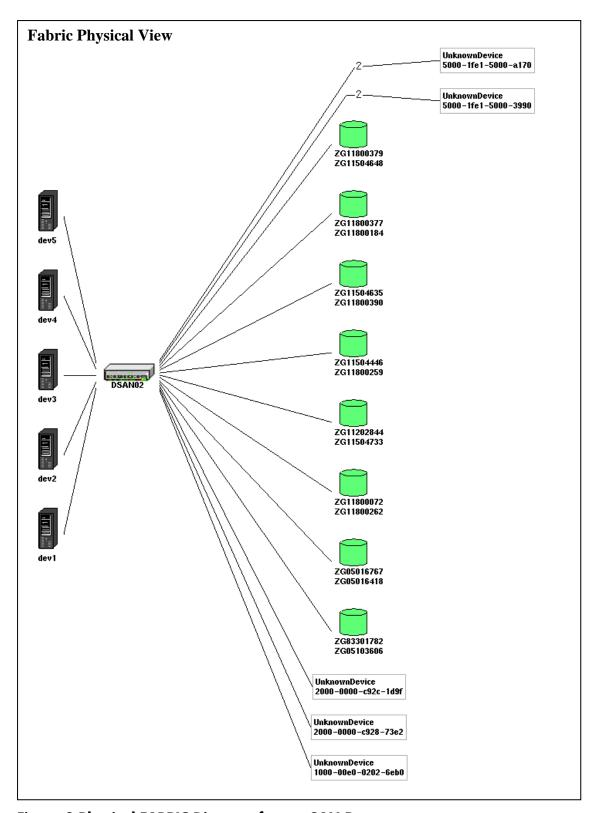
Figure 9 Physical FABRIC Diagram from a SAN Report
