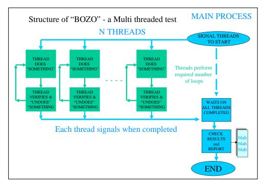
Figure 2 - Structure of a Multithreaded Test
