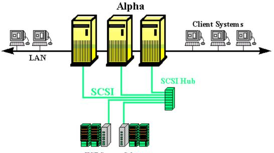
Example: SCSI-based OpenVMS Cluster using FWD HSZ Controllers
